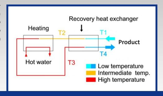
An electrically heated system is also an extremely economical option due to the high internal heat recovery rate of up to 95% (cold aseptic filling only). The internal heat recovery reduces the required steam or electrical output considerably. A heat recovery rate of 90% signifies that only 10% of the energy statistically necessary for heating up to the pasteurisation temperature is actually required. The higher the filling temperature, the lower the amount of energy recovered.
