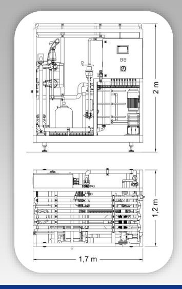
The pasteurisation is always subject to the contest between necessary temperature treatment and prevention of product damage (loss of taste). It is generally necessary to reach the pasteurisation parameters as quickly as possible, adhere to them precisely and then to cool down to ambient temperature as quickly as possible.
