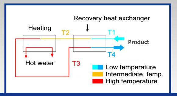
An electrically heated system is also an extremely economical option due to the high internal heat recovery rate of up to 95% (cold aseptic filling only). The internal heat recovery reduces the required steam or electrical output considerably. A heat recovery rate of 90% signifies that only 10% of the energy statistically necessary for heating up to the pasteurisation temperature is actually required. The higher the filling temperature, the lower the amount of energy recovered.
