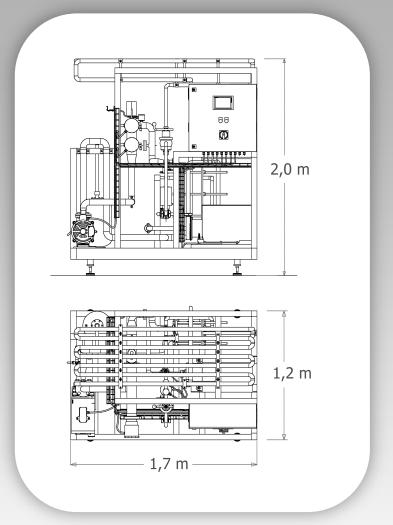
A pasteurisation temperature of 75°C and a heat holding time of 30 seconds are normally applied for milk. As pasteurisation at 95°C is possible with our MiniFlash system, the system is suitable for a wide range of milk products. Products with a viscosity of up to 500 mPas can be processed without any major modifications.
